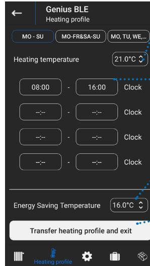
Determine the heating temperature with which the heating is to be carried out during the heating periods
