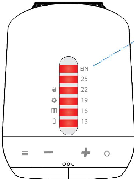
All 6 LEDs on: > 28° = heating ON (valve fully open, no regulation)
