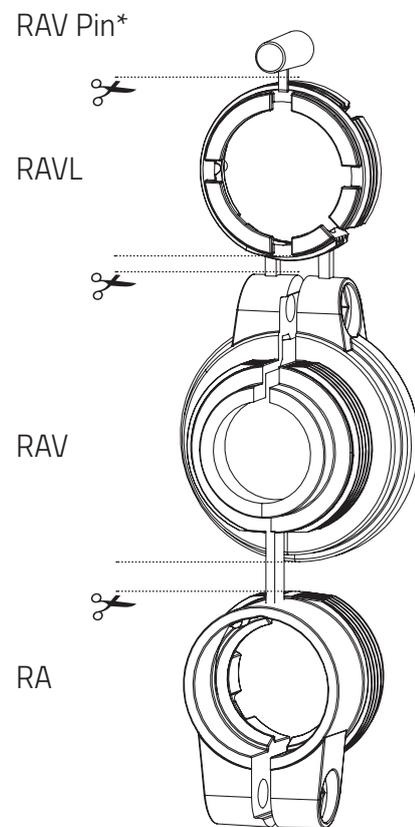
\* When using the RAV adapter, you need the RAV Pin for the extension of the valve stem.
