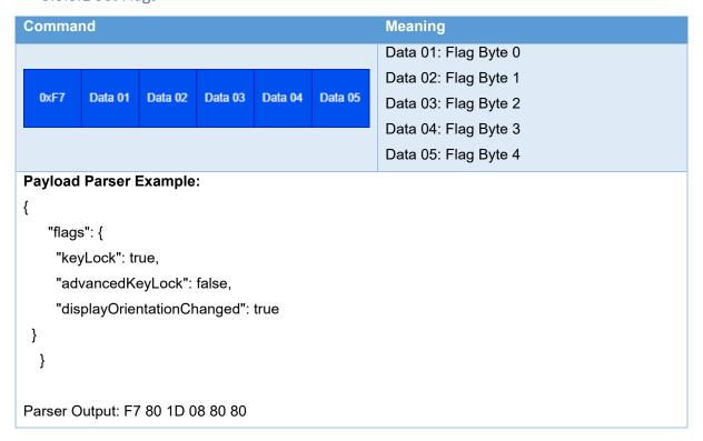
If child protection or display orientation should be changed the whole flag package must be sent. It is not allowed to enable child protection and child protection plus to the same time.
