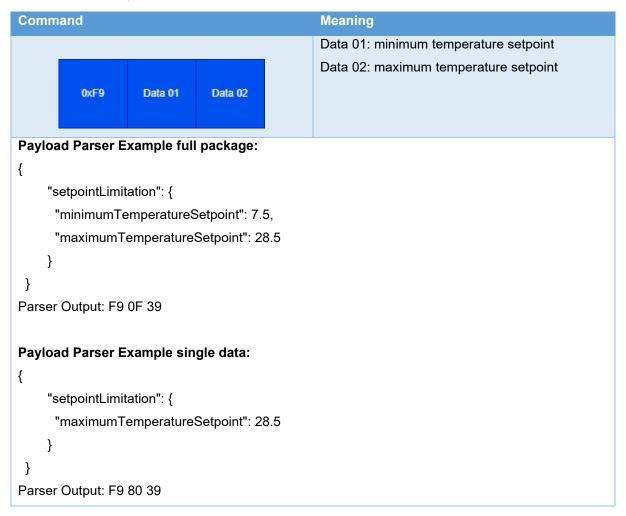
The following table shows the structure of the set setpoint limitation payload:
