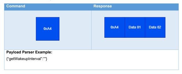
The following table shows the structure of the get wakeup interval payload:
