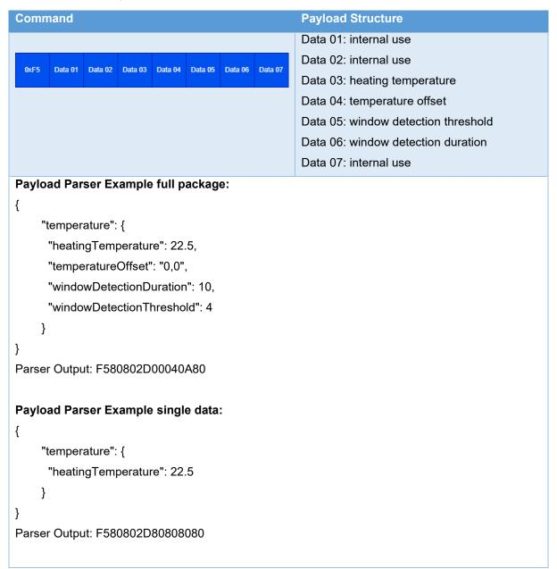
The parser allows to change single or multiple data.
