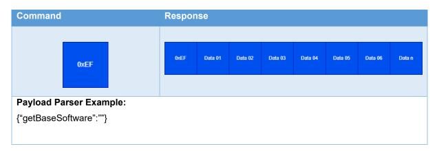
The following table shows the structure of the get base software payload:
