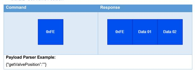
The following table shows the structure of the get valve position payload:
