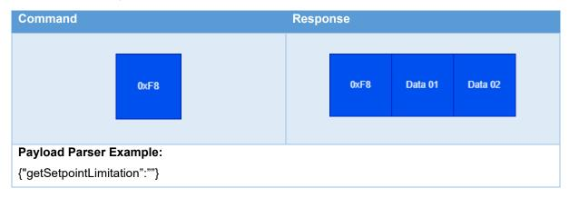
The following table shows the structure of the get setpoint limitation payload:
