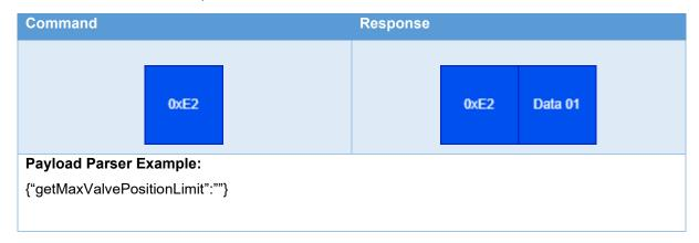
The following table shows the structure of the get max valve position payload:
