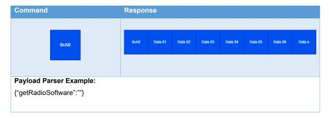
The following table shows the structure of the get radio software payload:
