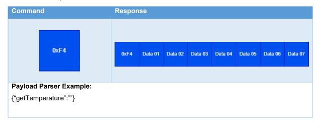
The temperature package contains of 7 data bytes. The following table shows the structure of the get temperature payload:
