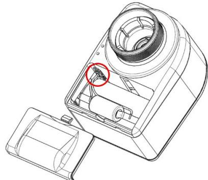
The Stella Pro LoRaWAN is powered by a lithium battery (3.6 V, C cell). This is equipped with a High Load Connector (HLC). The battery is connected to the plug in the battery compartment using the cable provided on the battery. Please ensure that the connection is correct before the device gets into use.
