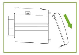
1. Press the battery compartment cover upwards and remove it.
