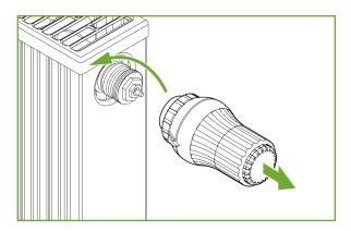
**1.** Open the current thermostatic head completely. Loosen the fastening and pull the thermostatic head off the radiator.
