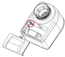
The Stella Pro LoRaWAN is powered by a lithium battery (3.6 V, C cell). This is equipped with a High Load Connector (HLC). The battery is connected to the plug in the battery compartment using the cable provided on the battery. Please ensure that the connection is correct before the device gets into use.
